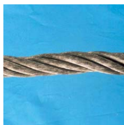
Reduction in wire rope diameter (hollowstand)
